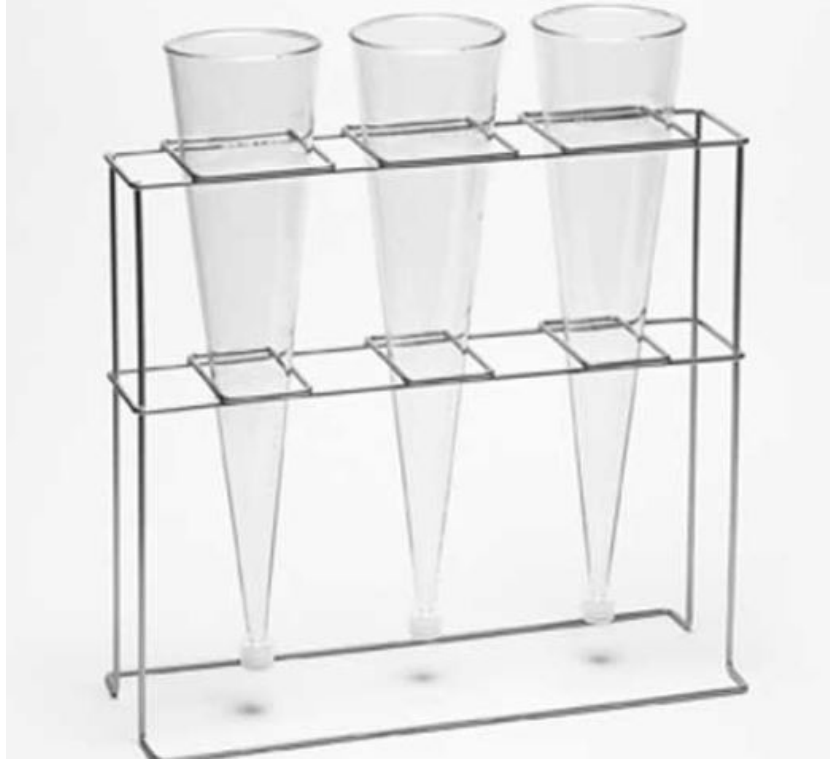
Image 5- example of Imhoff Cones used in Part III of laboratory assignment
